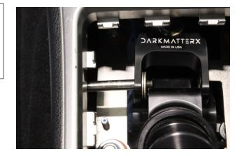
Align the top throw selection holes on the shifter with the bolt and washers, and push the bolt through just enough to place the next washers on the passenger side.
