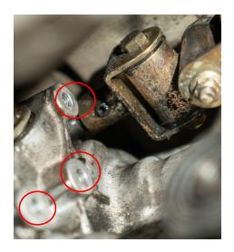
Place the punch directly over the roll pin and drive it out completely by tapping a hammer on the punch. If the roll pin is having a hard time coming loose, try soaking it in penetrating oil. This can help break it free easier.
