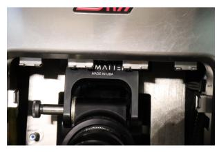
Gently insert the last (2) washers ensuring they do not drop, and finish pushing the shoulder bolt all the way through the shift arm. The threads should be sticking out on the passenger side and the bolt head should be flush against the shift arm
