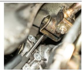
Once the roll pin has been removed, set it to the side as it will be re-installed back onto the vehicle.
