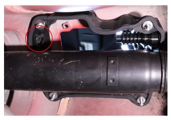
Insert the DM-2 back into the transmission tunnel.
