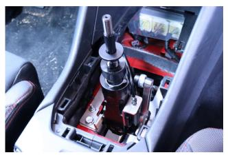
Disconnect the OEM shift cable from the DM-2 by removing the OEM cable hanger bracket and pulling the hitch pin from the cables connection point on the DM-2. Rotate the DM-2 counter clock wise so that it can be pulled out of the transmission tunnel.
