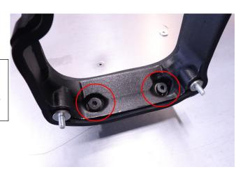
Insert the Main Flange above the driveshaft and use a 5mm allen wrench to secure the (2) bolts into the chassis of the car.
