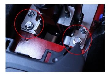
Next, locate the (2) supplied M8X1.25mm bolts from the hardware kit. These bolts will replace the front (2) mounting bolts that were previously removed. These bolts are longer and will allow the Main Flange to be secured.
