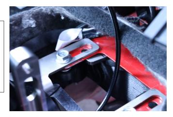
The bracket can now be fully tightened with its original hardware. Ensure the bracket keeps parallel alignment with the main flange.
