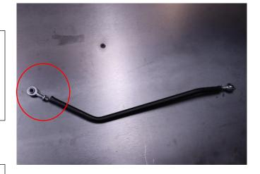
Re-install the rod end back onto the shifter and adjust it into place. Tighten the jam nut when put into place.
