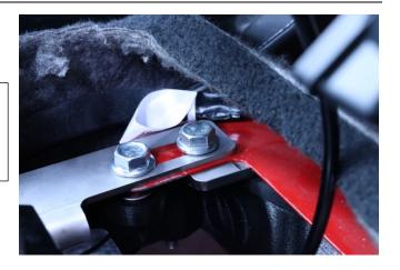
Install the (2) supplied M8X1.25mm nuts from the hardware bag to finish securing the main flange.
