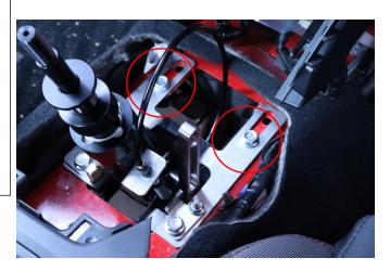
Locate the OEM cable holder bracket.
