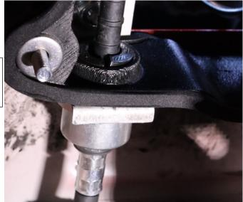
Install the OEM cable onto the shifter. It is crucial that the cable slips directly over shifter with out being tensioned or compressed. If it does not slip straight onto the shifter, then an adjustment will need to be made. To re-align the two components. The DM-2 install guide outlines how to adjust the large plastic piece at the end of the OEM cable into place. Another option could be to move the OEM cable hanger bracket slightly forward or back.
