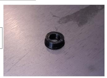
There is a slot on one section of the grommet that will allow the OEM cable to pass through it. Orient the grommet so that the flanged side is facing the front of the vehicle.
