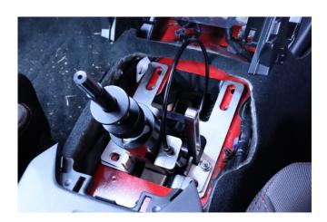
Insert the same (2) M8X1.25mm mounting bolts back into the Rear of the DM-2. Keep these bolts loose for now, so that the DM-2 can still be moved around.
