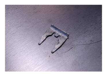
Re-install the OEM cable clip with the flanged edge facing the front of the vehicle.
