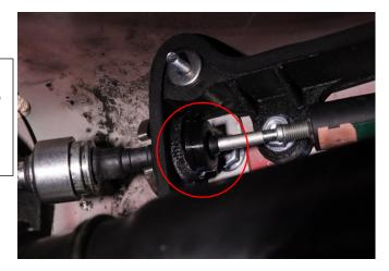
The grommet can be pushed into the box to form a tight seal against the cable. Start by pushing in one side first, and then working your way around until it is nearly flush with the main flange.
