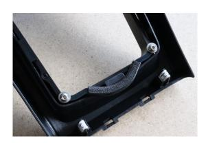
Place the front edge trim and front bracket together, with the interior lip of the edge trim facing away from the trim. Use the M6x16mm stainless bolt and place it through the front bracket with the stainless steel washer going in between the bracket and the trim. When tightening the bolt, it can help to hold the bracket with a pair of pliers to ensure it stay in the proper orientation.
