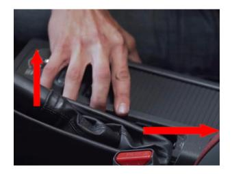
Remove the shift knob off of the shifter. Using both hands, remove the section of interior trim that is surrounding the shifter and has the shift boot attached to it. Working from the edge closest to the back of the car, gently pull up and continue this motion across the edges of the trim until it becomes free.
