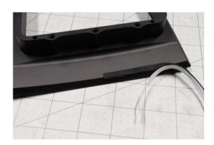
The foam should follow the flat edge on the bottom side of the trim, and can be placed by first peeling the paper off the side of the foam covering the adhesive.
