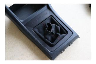
Install the interior trim back into the vehicle and resecure the center console back into place.
