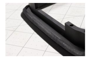
Locate the rear bracket and edge trim and place the edge trim over the bracket. Note that there is a lip on one interior side of the edge trim. This side with the lip should be facing away from the trim when installed.
