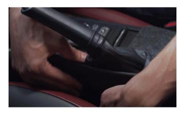
Firmly pull up on the front of the center console until it comes free. Push the console towards the back of the car a few inches so that you expose the area behind the shift boot trim.
