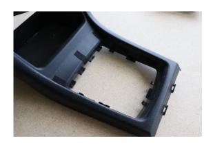
Locate the foam provided in the kit and place it around the perimeter on the bottom side of the billet trim.
